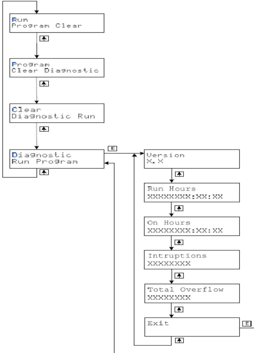
Current Firmware Version, On and Run Hours can be viewed. On Hours inform the time for which Flowmeter is on and Run Hours indicate the Flow Hours. INT indicate Power Fail Interruptions and T OF indicate numbers of Totaliser overflow.
